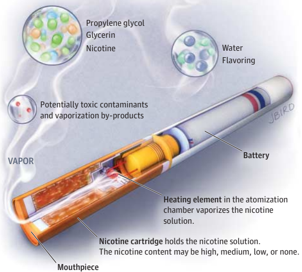
Parts of an e-cigarette structure and substances that may be found in the vapor
